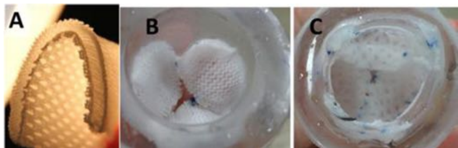
Figure 17. Three-dimensional weft-knitted spacer fabric made out of PET yarn, originally made for sport-garment.
